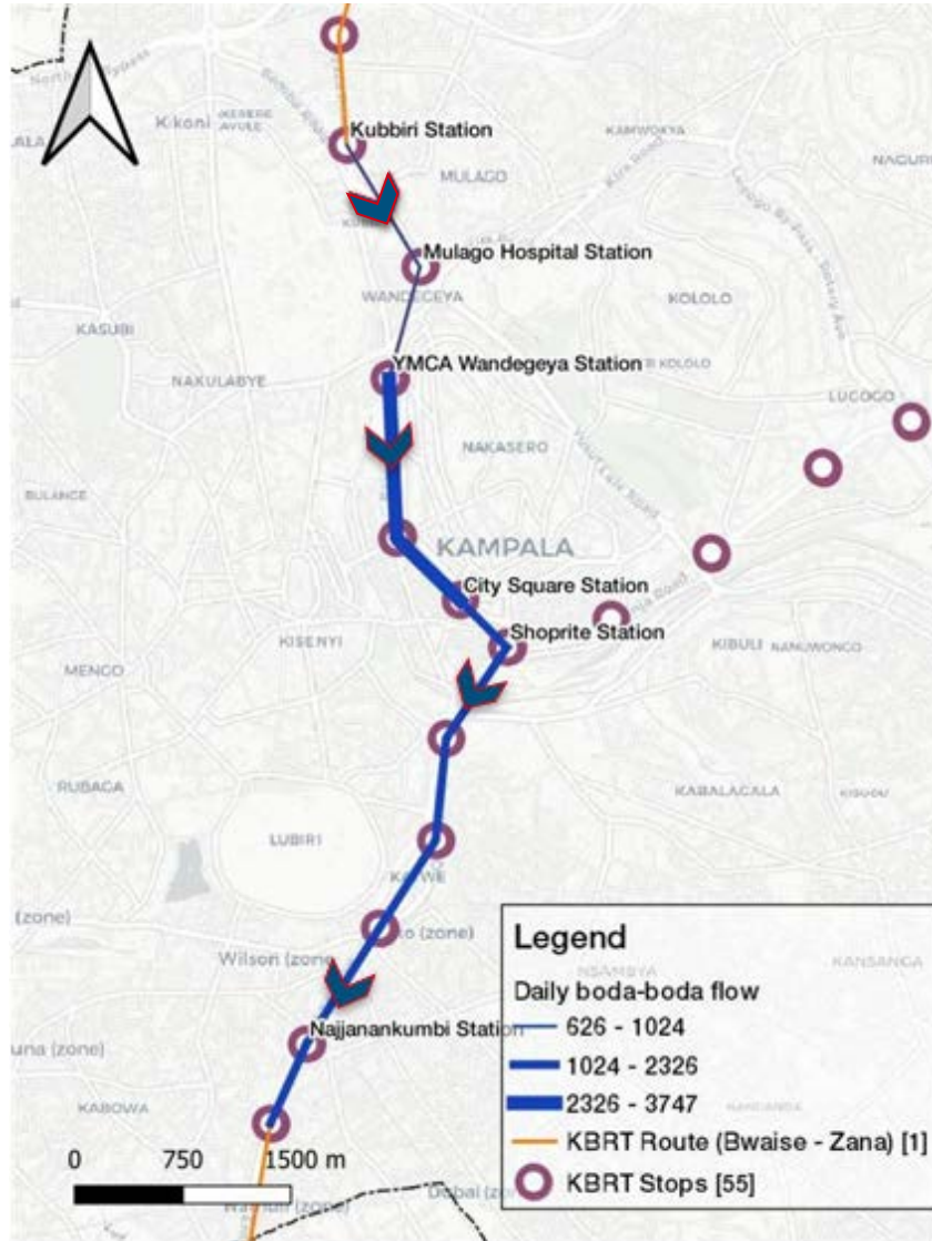
Figure 6 Hourly boda-boda flow in the BRT 3 line in the direction of Bwaise to Zana
